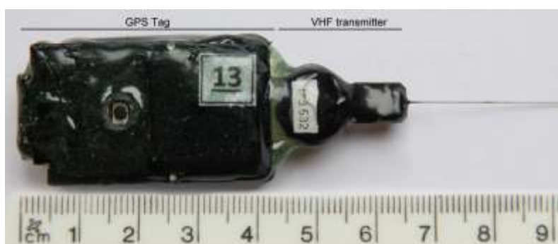
Figure 5.9 The GPS tag with the smaller Titley LT5-357 VHF transmitter attached. The combined package weighed 22g and was 65mm long (excluding 14cm flexible trailing whip aerial). During field use, waterproof tape covered the operating button in the centre of the GPS tag.
