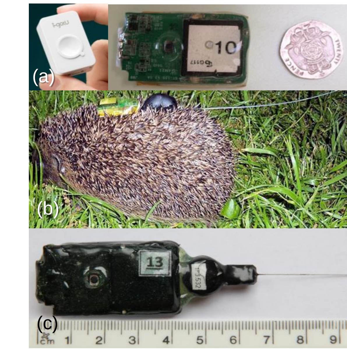
Fig.1. (a) GPS tag pre- & post- modification. (b) GPS & Biotrack VHF tags in use. (c) GPS tag + Titley VHF tag glued together.
