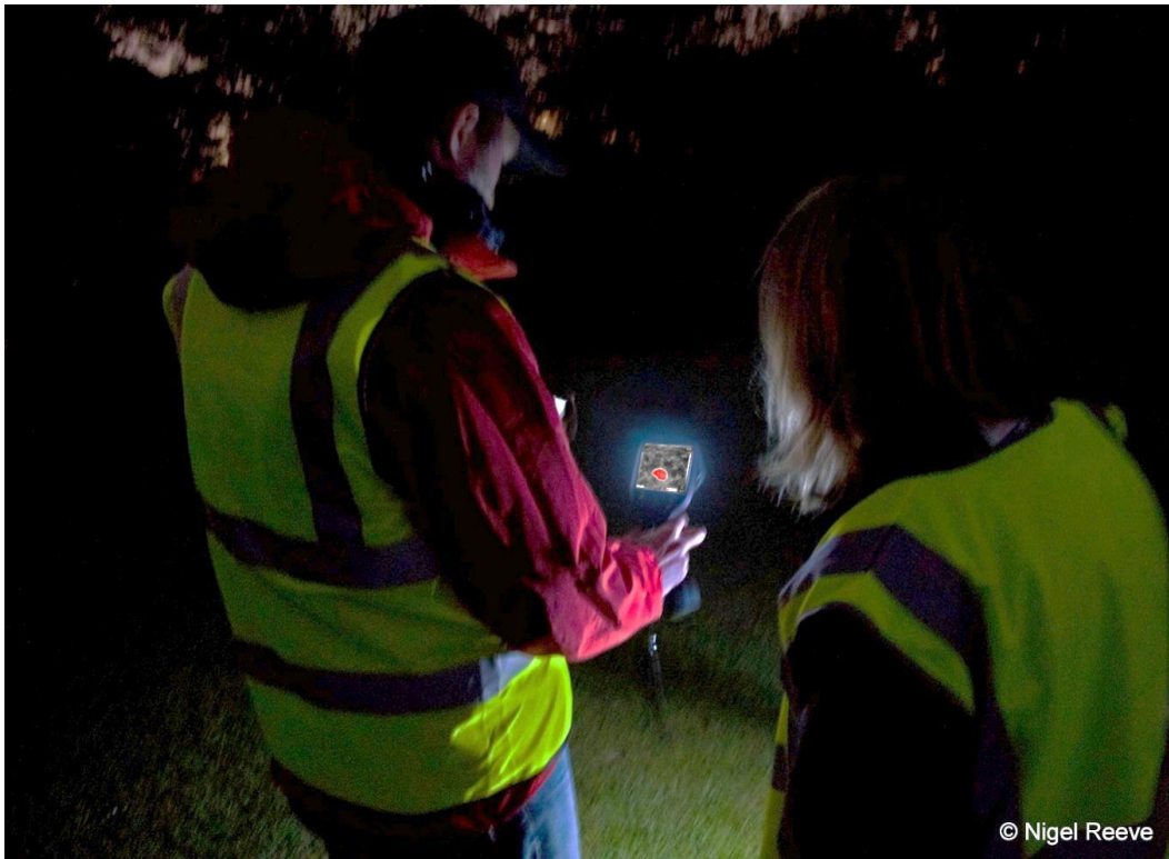
Figure 5.2 The FLIR E60 in field use with display set in 'Alarm mode' for behavioural observations during 30minute sampling periods. .
